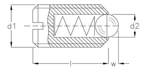
$\begin{array}{ll} d1 & = M10 \\ d2 & = 6.0 \\ I & = 19 \\ Spring \ pressure \ N \ bottom = 45 \\ Spring \ pressure \ N \ top & = 20 \\ W & = 2.0 \end{array}$
